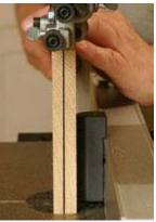
The full-featured T-square style fence (left) locks on both ends for maximum stability. The resaw post (right) is included and attaches to the fence with a finger knob.
